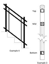
Position rails against posts and even the end spacing on each end, if possible, with balusters parallel to the post. Clamp rails to post (Example 4). Mark rails for cutting (Example 5). Mark posts for each mount position (Example 6). Cut rails and vinyl inserts 3/16" shorter than mark on each end. Rails should be cut using a straight cut.
