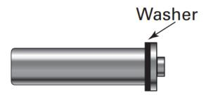
2. Rotate the Pull-Lock® fitting clockwise as you push it onto the cable. If the cable begins to "unravel," you are rotating the fitting in the wrong direction.
