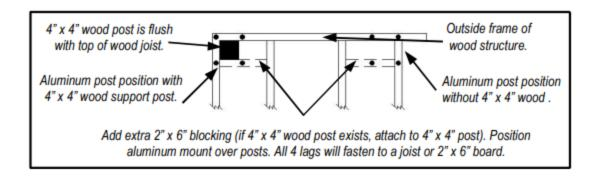
b. For IRC wood surface installation; attach wood blocking to substructure with #10 x 3" wood screws. Fasten aluminum post using (4) 3/8"x 5-1/2" bolts (anchors not included) thru aluminum backer plate (sold separately) as shown below.
