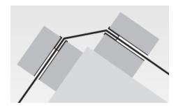
Double-Post 90<sup>0</sup> corner illustrated without the Corner Kit installed, showing the cable assembly passing through each post with Isolation Bushings at directional changes.
