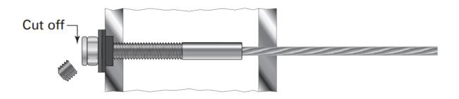
2. Twist the cap over the locknut.
