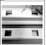
8. From the centerlines marked on both the Top Rail and Bottom Rail in step 7, place a mark 1/2" to the left of the centerline on the Top Rail (A) and 3/8" to the right of the centerline on the Bottom Rail (B). These marked locations will become the new centerline mark of both rails to determine cutting locations.
