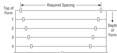
Figure 1 — Spacing Locations (side view)
