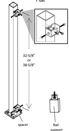
4. Fasten rail support to bottom side of bottom rail by inserting pan head self-tapping screw (provided) through center of threaded portion of support. This applies to all sections over 6ft long.
