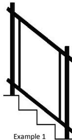
4. **Crossover Railing:** For crossover stairs set stair crossover kit next to rails that are fastened to post to determine what height to cut post. Mark post and cut. Set crossover connector in post and fasten at proper height with self-tapping pan head screws provided. Set correct angle for crossover connector to match railing and tighten nut. Cut bottom rails same as above in step 3 (Example 3). Mark top rails to cut making sure it fits snug into the crossover connector (Example 4).
