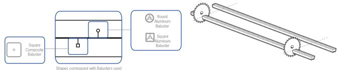
Use the shape guides printed on the underside of the Universal Rail with the corresponding Baluster to determine where the Balusters will be placed, before cutting the Universal Rails. The spaces between the Baluster will be less than 4".
