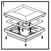
1. The following components are included with the FortressAccents 3.5", 4" and 5" Flat Pyramid Caps: Post Cap, Post Cap Base, Light Slot Cover, 4 - Machine Screws, and 4 - #10 X 3/4" Wood Screws. Note: 5" Flat Pyramid Caps include a Composite Adapter with 4 - Pan Head Machine Screws.
