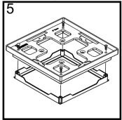
5. If installing FortressAccents 5" Flat Pyramid Post Caps on Composite Posts wider than 4.5" the Composite Adapter will need to be removed. With Composite Adapter removed the 5" Flat Pyramid Cap will fit posts up to 5" in width.
