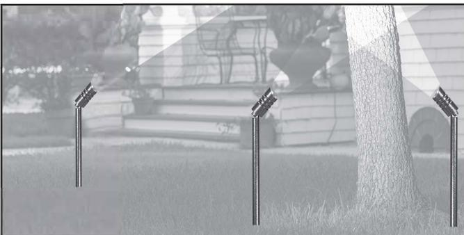
2 Place all lights in desired location. If necessary use 3/4" (1.9 cm) auger with in a drill to penetrate the surface enough to ensure the fixture is firmly implanted. (See warning on Page 1).
