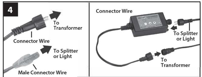
4. Connect all lights. Then connect the optional dimmer (recommended) between the main 20' (6.1 m) transformer male to male lead and the transformer for each circuit. Make sure connections, fixtures, and power sources (including splitters) are all working.
