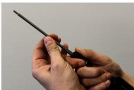
Pull the chuck back to allow the bit to pull free and install the new bit.
