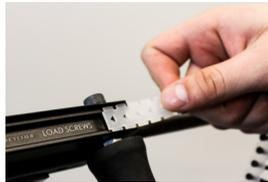
Slide strip into screw strip channel
