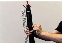
Hold body of the tool with one hand so that screws stay in place
