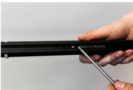
Use a bit to depress the release button in the channel.
