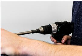
To attach to a tightening chuck, simply insert the large collar of the drive shaft into the drill chuck and tighten
