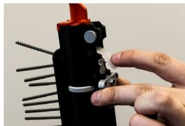
Slide picker up to nose of the tool and fold the open strip onto the picker teeth with your pointer finger
