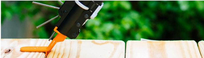
Using the Tool Handle, apply downward pressure to make sure that the nose stays firmly in position with the board edge throughout the drive process.
