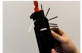
Slide collation strip up and through the nose of the tool until it will go no further
