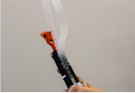
Slowly return the picker to the bottom of tool. Caution! Be very careful not to let go of the picker as it will recoil very quickly and could damage the tool when it strikes the stop.
