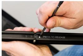
As you depress the release button, remove the lower body of the tool.
