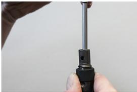
Take an extra CAMO® DRIVE™ bit and insert into the end of the collar
