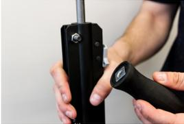
The handle is attached to the tool body screwing it onto the bolt found installed at the top of the tool body.
