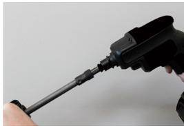
Attach your driver drill's locking chuck to the smaller bit
