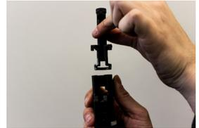
Insert new guide paying attention to the direction of the alignment tabs.
