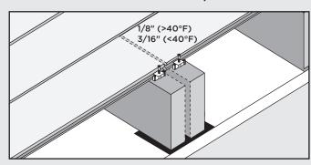
**NOTE:** Optional - Gap joist framing 1/8" - 1/4" to allow for water drainage.
