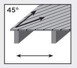
At a 45° angle, maximum joist spanning is 4" (102 mm) less than listed in the chart below.
