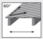
At a 60° angle, maximum joist spanning is 2" (51 mm) less than listed in the chart below.
