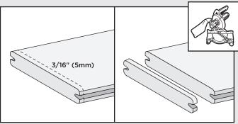
It is recommended that boards be clean cut on both ends a minimum of 3/16" (5mm).
