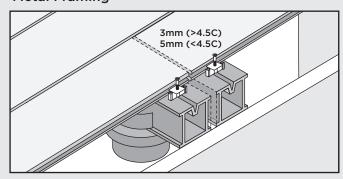
**NOTE:** Hidden Fasteners MUST be used at every joist.
