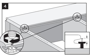
**NOTE:** Use scrap piece of decking to help hold fastener in place while attaching.
