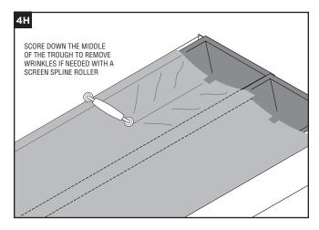
**NOTE:** In extreme temperature swings, trough material will expand and contract. Some wrinkling is acceptable but should not impede the flow of water.
