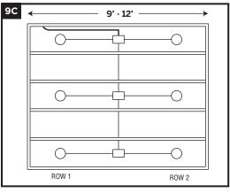
EXAMPLE OF A 3 ROW LIGHT INSTALLATION FOR JOISTS BETWEEN 13' AND 16' (3.96 - 4.87 M)
