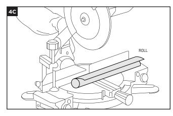
»Measure over 4" on the 1-1/2" score mark side and cut off for 12" on center joists. (4C)
