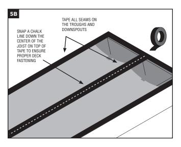
**NOTE:** The butyl tape should never be put directly on the board without the trough material or a downspout below it.
