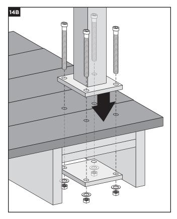
»Attach posts using four 3/8" x 6" (1 cm x 15.2 cm) hex cap bolts, washers, and nuts, along with aluminum back plate on underside of blocking.
