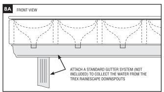
**NOTE:** Installing a clean-out trim piece will allow access to gutter line after installation.
