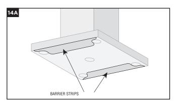
»Insert the (2) stainless steel barrier strips under the mounting bolt holes. Barrier strips are required only if attaching post directly to pressure treated framing.
