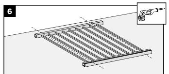
6. Cut panel use a reciprocating saw (equipped with a metal blade).
