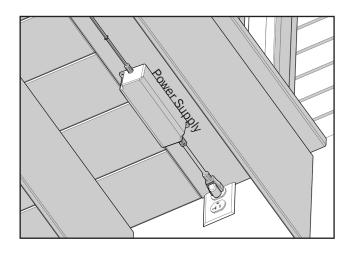
The Power Supply can be mounted under the deck, and out of sight. With an IP67 Waterproof rating there's no need to worry if it gets wet. It is our recommendation that a "drip loop" be created during wire routing. Below is an image of how to properly orient the wires.
