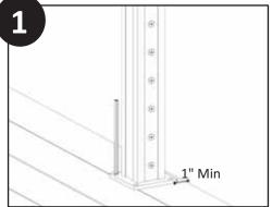
Measure & mark post placement evenly. Set each post with minimum of 1" from the edge of the post plate & deck or step. Mark each hole in the post plate on the deck or step for bolt placement.
