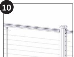
Using the provided needle connected to the end of each cable, insert each cable through it's hole in each baluster and channel in each line post.
