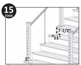
On stairs use the post with greater spacing to the bottom receiver for the bottom post. Standard posts can only be used on stairs when rise is 7-1/2" and run is 11". For any other dimensions, blank posts will need to be used and custom drilled
