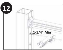
Using the cable vise grip, insert each cable a minimum of 1-1/4" into each end post receiver.
