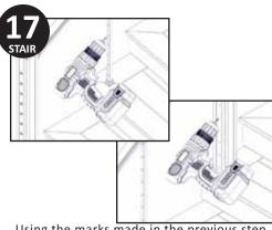
Using the marks made in the previous step, drill 3/16" holes aligned with each mark on each line post and baluster at the angle of the stairs.
