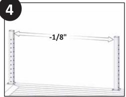
Measure the distance between connecting faces of posts. When measuring a stair section measure at the angle of the stairs.
