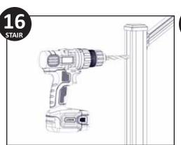
For nonstandard stair sections, align a string with each hole in the top post &, keeping it the same distance from the nose of each step, run the string to the corner of the connecting face of the bottom post, marking the bottom post & each line post & baluster. Use each mark on the bottom post to drill a 17/32" hole through the front and back of the bottom post.
