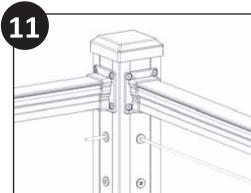
Insert each cable through it's channel in each corner post. This will require more force than the line post channel insertion.
