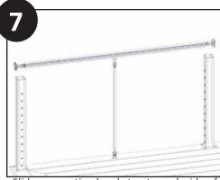
Slide a mounting bracket onto each side of the top rail. Set the baluster in the bottom baluster mount then lower the top rail into place ensuring the top baluster mount envelopes the baluster.
