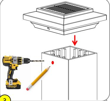
Place the solar Post Cap on the post. Mark both holes on the post. Use an appropriate drill bit to make a small pilot hole for the provided screws.
