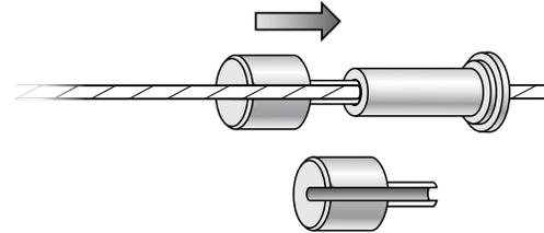
Insert the shaft of the tool into the end of the Quick-Connect® fitting and push firmly to release the jaws. While maintaining pressure on the tool, remove or reposition the fitting as needed. The jaws will automatically re-grip the cable when the tool is removed. Note, if the fitting has a silicone Protection Seal, remove seal prior to inserting the tool.
