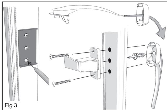
F: Install appropriate strike for adequate latching
