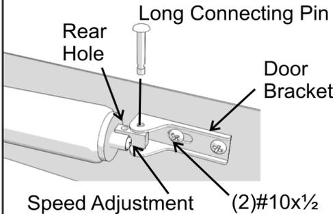
**C2:** After installing the door bracket, return the "Hold Open Washer" to the normal position.
