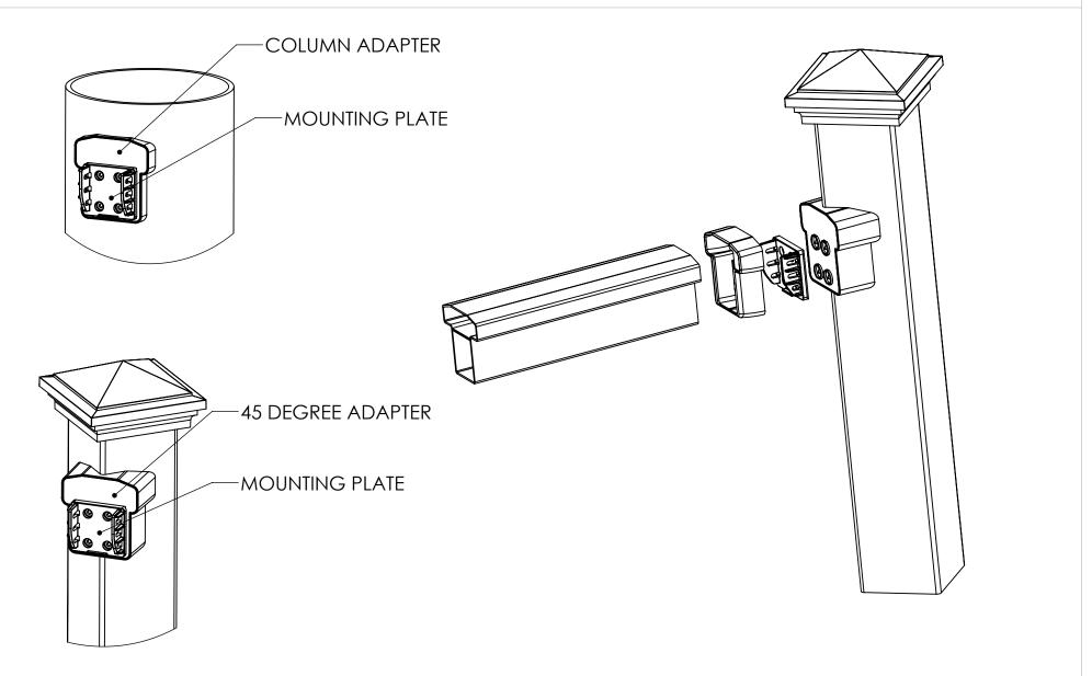
A 45 DEGREE OR A COLUMN CONNECTION CAN BE ACHIEVED BY PLACING A MOUNTING PLATE INTO THE DESIRED ADAPTER AND FOLLOWING THE SAME PROCEDURES AS THE STRAIGHT BRACKET INSTALLATION.
