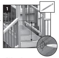
**NOTE:** If deck boards are not installed yet place an appropriate deck width spacer board to ensure post sleeve is at correct height.
