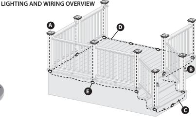
NOTE: All wiring and splitters are mounted to inside of framing, picture is just representation of where to place these in general.
