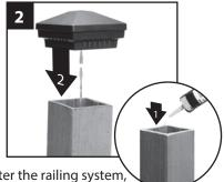
**NOTE:** Install post cap lights after the railing system, post sleeve skirt, and post sleeve have been installed.
