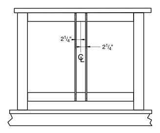
**Step 3:** Use a section of 2x4 to space the next baluster 3-1/2" from the first. Attach the rest of the balusters using the 2x4 as a spacer block. Cut two support blocks from the wood or composite railing material you're using. Glue support blocks to the bottom of the lower rail an equal distance from each post.
