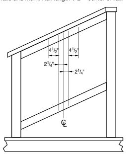
**Step 2:** The baluster spacing is 4-1/2" on-center and equal spacing for the end spacing. For posts set at 6' on-center, attach the first two balusters 2-1/4" on-center each side of the center line using four of the screws provided. Use the plastic washers when using treated lumber, to prevent direct contact. Place the washer in between the rail and baluster.
