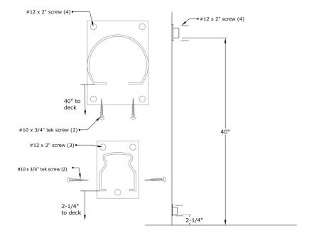
Wall brackets can be used to attach top and bottom rail to existing wood posts or walls. To locate the bottom wall bracket, measure up 2 1/4" from deck to the bottom of bracket as shown in drawing. To locate the top wall bracket, measure up 40" from deck to the bottom of the top bracket as shown in drawing. Secure with supplied screws. To mount wall brackets to aluminum posts, secure with #10 x 3/4" tek screws. (not supplied)
