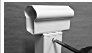
4. Position the post(s) on the flooring surface based on the project layout described in steps 1 & 2. Mark the locations of the four (4) 3/8" diameter holes provided on the mounting flange, and remove the post. Drill the marked locations into the flooring surface material and fasteners being used. Reposition the post in the location that has been marked and drilled, and secure the post mounting flange to the flooring surface making sure post(s) are plumb.
