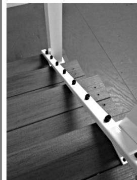
2. When the final position is determined for the post, mark the hole locations of the four 3/8" diameter mounting holes provided on the base and remove the post assembly. Drill the marked locations into the decking and reinforcement using the proper size drill required for the fasteners being used.
