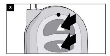
Press and hold both the up and down arrow on the dimmer remote simultaneously.
