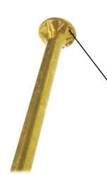
The head has a 90° angle at the underside which allows it to fit perfectly into the pre-countersunk holes of hardware fittings such as hinges or locks.
