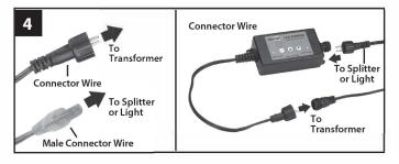
Connect all lights. Then connect the optional dimmer (recommended) between the main 20' (6.1 m) transformer male to male lead and the transformer for each circuit. Make sure connections, fixtures, and power sources (including splitters) are all working.
