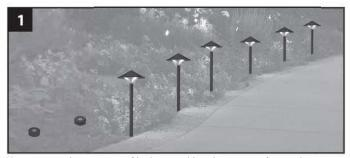
Locate placement of lights and lead wiring. If you choose to bury wire, under concrete or other permanent structures, plan accordingly.
