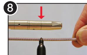
8 Stretch cable tight across fitting and mark at Cut Gauge Line. Cut cable at mark.
