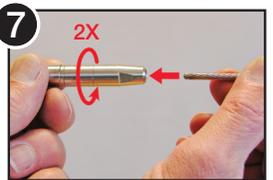
7 Loosen Quick-Connect® 2 full turns and insert cut cable end as far as it will go into the fitting; the jaws will automatically lock on.
