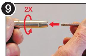
9 Loosen the swivel component 2 full turns and insert cut cable end as far as it will go into the fitting; the jaws will automatically lock on.
