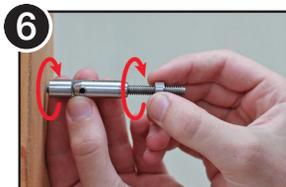
6 Spin the pivot component all the way onto the hanger bolt. Make sure the lock-nut is all the way on the threads.
