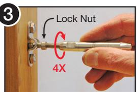
3 Spin the turnbuckle lock-nut onto the exposed threads. Then attach Quick-Connect® and rotate the body 4 full turns.
