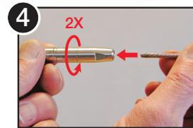
4 Loosen Quick-Connect® 2 full turns and insert cut cable end as far as it will go into the fitting; the jaws will automatically lock on.
