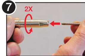
7 Loosen the swivel component 2 full turns and insert cut cable end as far as it will go into the fitting; the jaws will automatically lock on.
