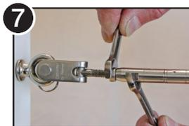
7 Tighten the lock-nut against the swivel component to prevent the fitting from loosening.
