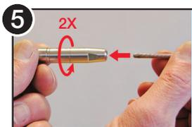
5 Loosen Quick-Connect® 2 full turns and insert cut cable end as far as it will go into the fitting; the jaws will automatically lock on.
