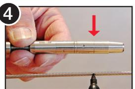
4 Stretch cable tight across fitting and mark at Cut Gauge Line. Cut cable at mark.
