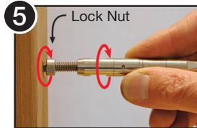
5 Spin the turnbuckle lock-nut onto the exposed threads. Then attach Quick-Connect® and rotate the body 4 full turns.
