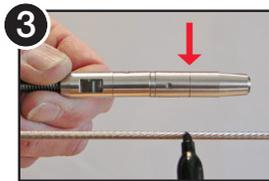
3 Stretch cable tight across fitting and mark at Cut Gauge Line. Cut cable at mark.
