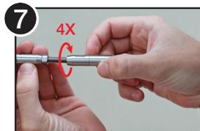
7 Attach the QC swivel component to the threads with 4 spins. Do NOT add the Locktite to these threads, or you will not be able to properly tension the cable.
