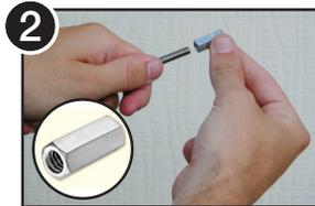
Spin Hanger Bolt Installation Tool onto the end of the bolt.
