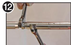
12 Tighten the lock-nut against the swivel component to prevent the fitting from loosening.
