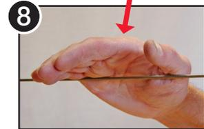
8 Hand tighten the turnbuckle as far as possible, then swiftly hit the cable line with your palm several times to ensure that jaws are securely seated.
